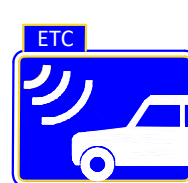
Fig.17.29 GUIDE SIGN ON TOLL LANE PORTAL
