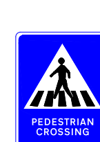
Fig.17.47 PEDESTRIAN CROSSING INFORMATORY SIGN
