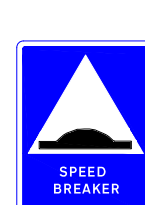
Fig. 17.48 Speed Breaker Informatory Sign
