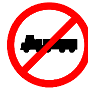
Fig. 14.15 Articulated Vehicles Movement Prohibited
