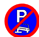
Fig. 14.33 Parking Not Allowed on Half of Footpath
