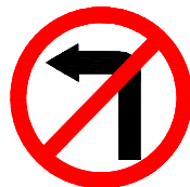
Fig. 14.23 Left Turn Prohibited
